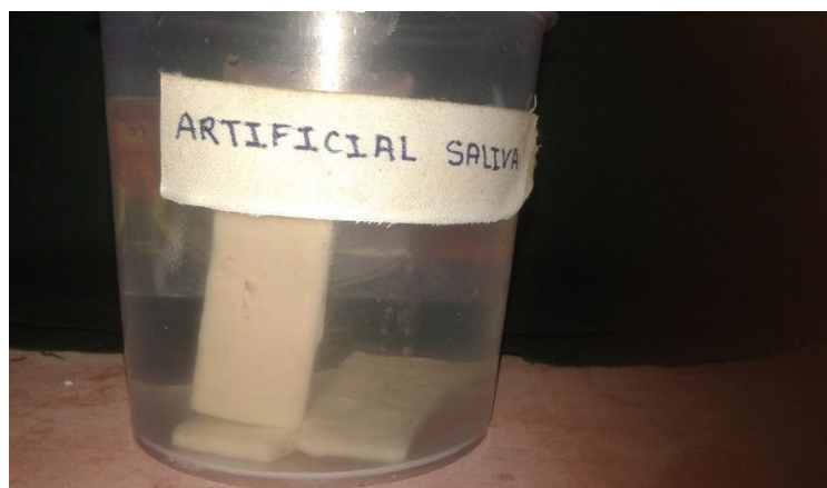
Figure 5: Samples stored in artificial saliva.
