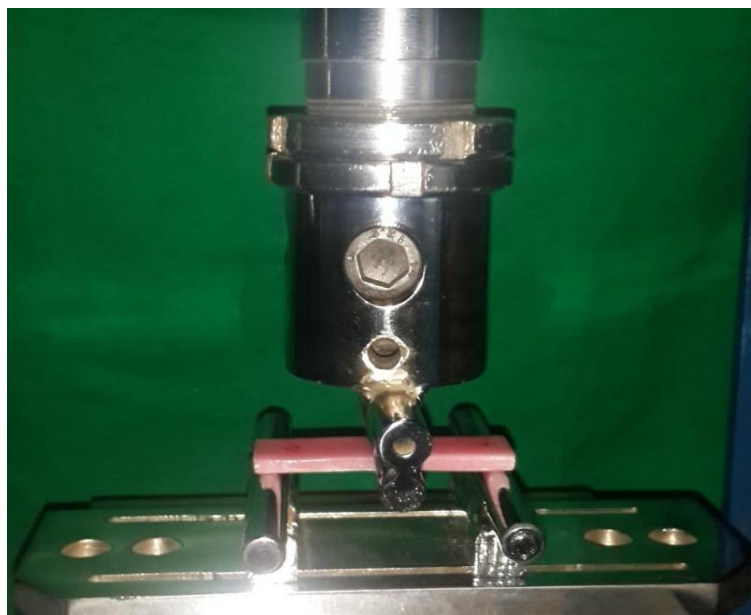
Figure 6 : Acrylic samples testing on Universal testing machine.
